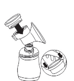
3 Place the silicone diaphragm into the pump body from above. Make sure it fits securely around the rim by pressing down with your fingers to ensure a perfect seal.
