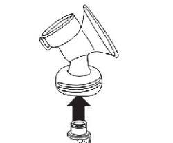
1 Insert the valve into the pump body from underneath. Push in the valve as far as possible.
